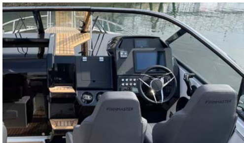
Yamaha full elektrisk styrning (SBW & DBW).
